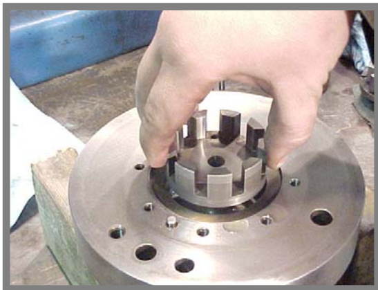
Rebuilding Oil Pump
